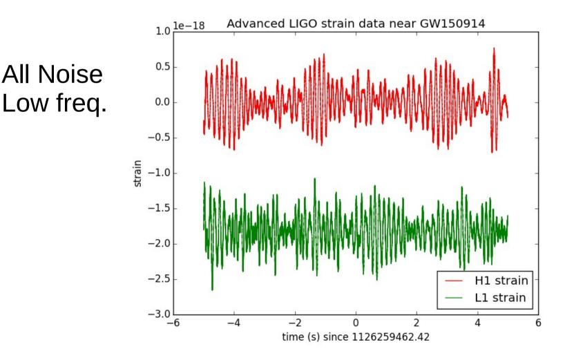
Filter out low frequencies (eg, oscillations of mirrors as pendula, laser pressure fluctn., shot noise, seismic,...) Filter out narrow line noise (eg 60Hz, 120Hz, 180Hz from powerlines, Filter out 500Hz string frequency of support wires, 10 calibration lines.
