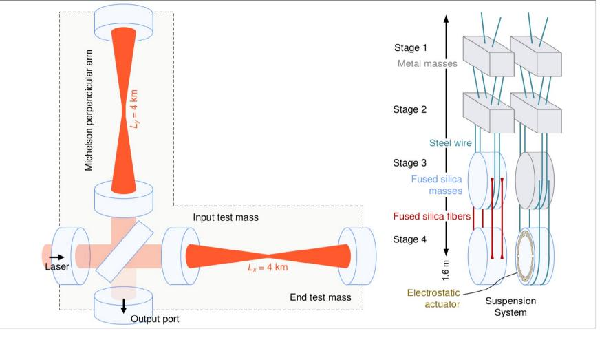
In operation, only tiny amount of light comes out to make sure both arms exactly the same length. Fluctuations in laser intensity do not come out the output but go back toward laser. (Common mode rejection).
