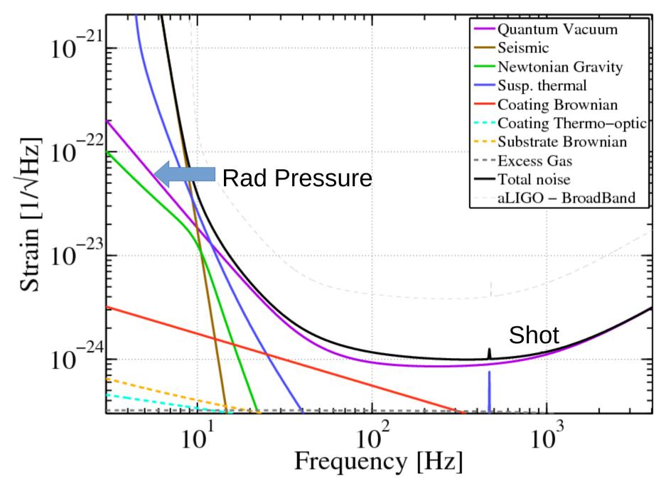
Quantum Noise dominates above the Seismic Threshold
