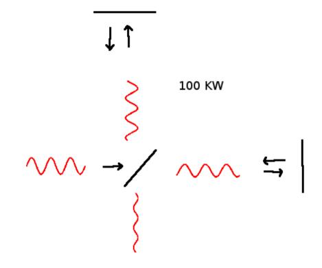
Crests and troughs line up in two beams. Cancellation at half mirror depends crucially on lengths
