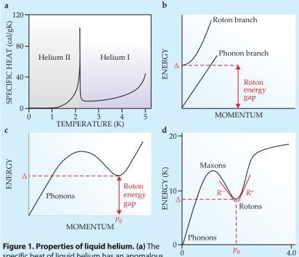
specific heat of liquid helium has an anomalous jump near 2.2 K. The "lambda transition" between
