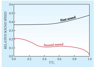
**Figure 5. Calculated first- and second-sound** velocities in a uniform superfluid gas of ultracold Fermi atoms at unitarity, the point at which the atomic scattering length is infinite. The velocities are given relative to the Fermi velocity, and the temperature *T* is scaled to the superfluid transition temperature  $T_c$ . (Adapted from ref. 13.)
