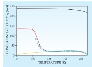
**Figure 2. The velocity of second sound** as computed by Evgeny Lifshitz (red curve) and by Laszlo Tisza (green curve); for comparison, the upper, black curve shows the velocity of first sound. The blue points are today's accepted values of secondsound velocity. Box 2 describes why Tisza's formula did not work.
