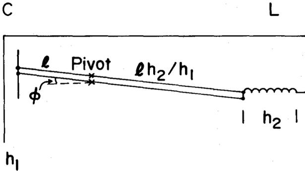
Fig. 5. Quantum non demolition readout of energy of electronic circuit coupled to mechanical bar.
