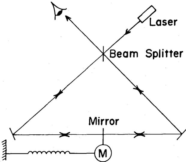
Fig 3. Laser interferometer readout of gravity wave detector.
