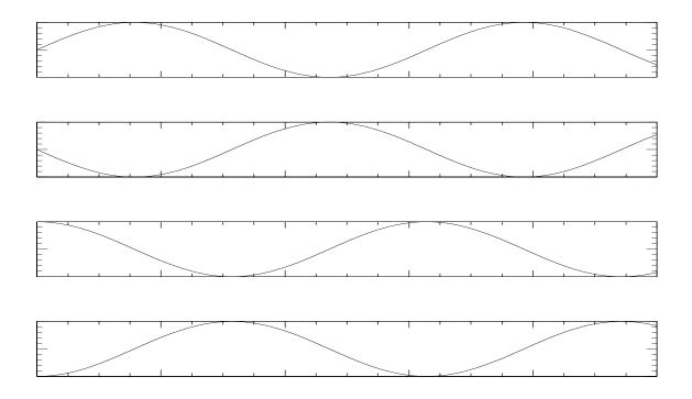
The phase shift is by what fraction of a cycle (multiplied by 360 degrees) one wave is shifted with respect to the other. If the shift is toward the future, (one wave "starts" after the other- ie has its maximum for example to the future- the shift is usually called positive. )
