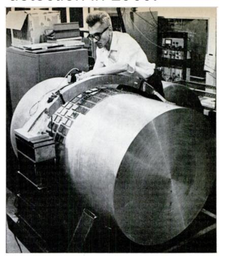
Over 1 ton aluminium bar vibration much less than an atom.
