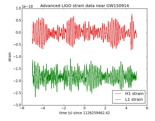
Filter out low frequencies (eg, oscillations of mirrors as pendula, laser pressure fluctn., shot noise, seismic,...) Filter out narrow line noise (eg 60Hz, 120Hz, 180Hz from powerlines, Filter out 500Hz string frequency of support wires, 10 calibration lines.
